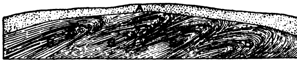
FIG. 88.—Diagrammatic section showing position of folded clays, State road, Dennis. A, glacial drift; B, folds in (Truro?) clays. 1 inch = 100 feet.
